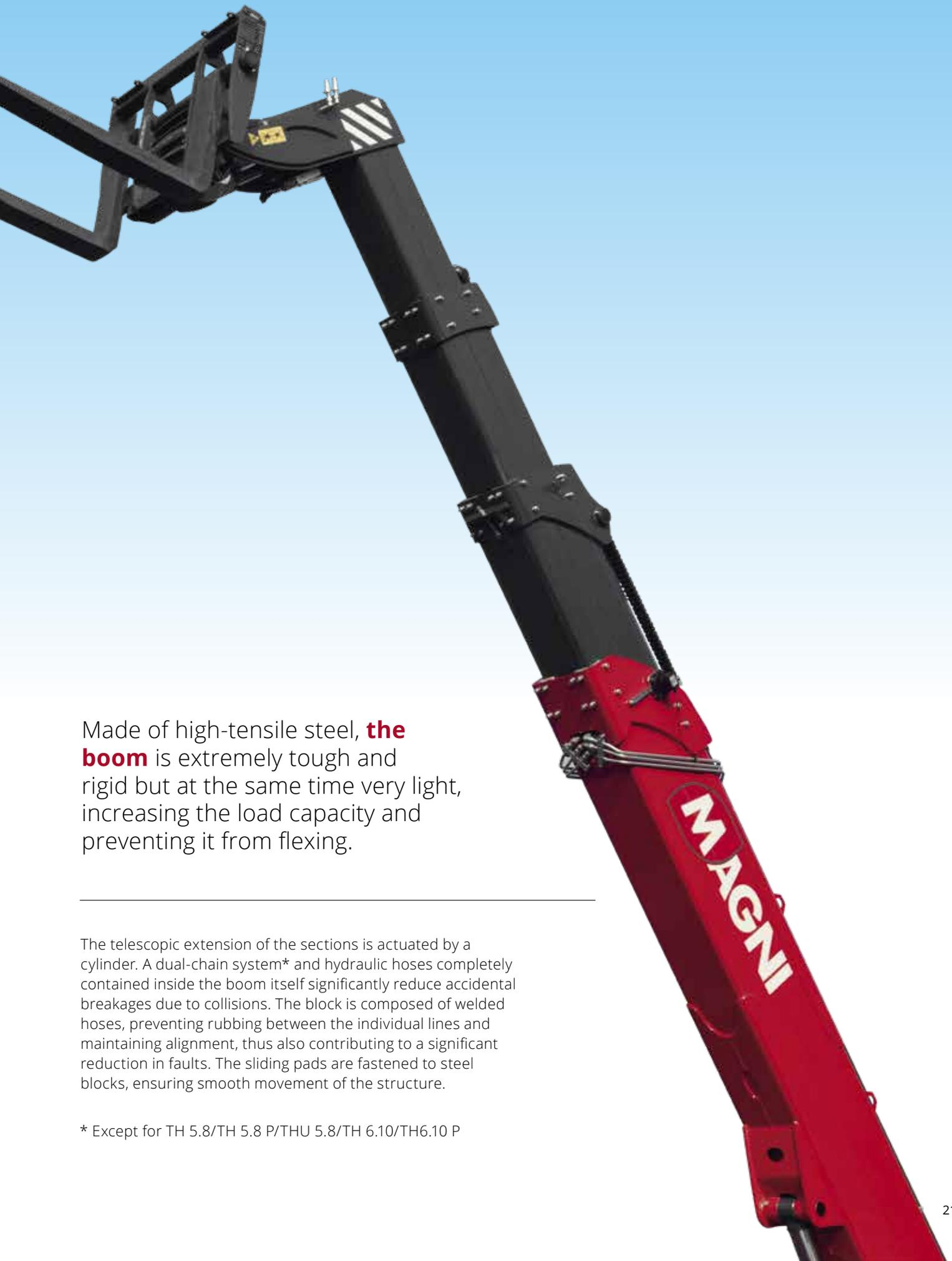
Made of high-tensile steel, **the boom** is extremely tough and rigid but at the same time very light, increasing the load capacity and preventing it from flexing.
