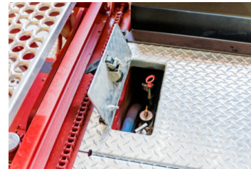
Daily Checks are Easily Accessed from the Operator Platform without Deck Lid Removal
