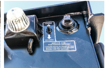
Service Cab Positioning Switch allows the Cab to be Traversed with Machine Powered Down
