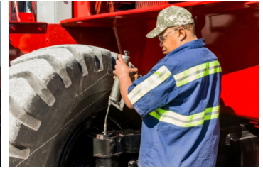
Easy Access for Steer Axle Maintenance
