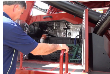
Service & Inspections from Running Board Dual Engine Bay Doors provide full access
