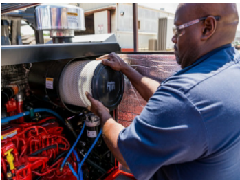
Donaldson Air Cleaner with Safety Element (Standard)
