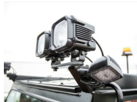
12 LED Work / Step Lights (Standard)
