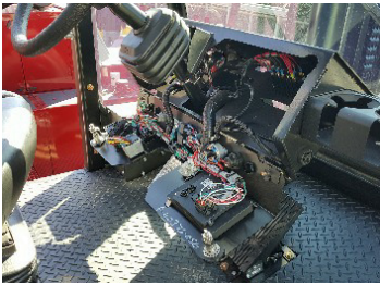
Flip-down Dash with Color/Number Coded Wiring (Standard)
