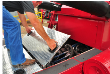
Lightweight Deck Lids Provide Easy Access to Hydraulics and Drivetrain
