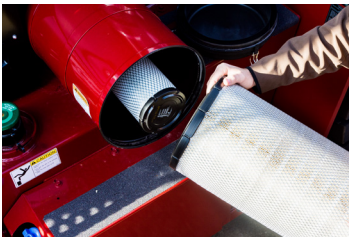
Donaldson Air Cleaner with Safety Element (Standard)
