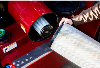
Donaldson Air Cleaner with Safety Element (Standard)
