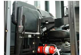
Fully Adjustable Mechanical Seat (Standard)
