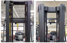
Nested I-beam mast rails provide the operator a wider view through the mast. Standard and multi-stage free-lift masts are available with lift heights up to 275-in.
