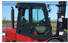
Full cabs with heat, defrost and optional A/C are available for max environmental comfort. Bi-fold doors lift off to provide open air cabin when needed.
