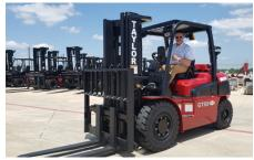
Working in containers introduces special height constraints. The available 87" reduced height overhead quard is purpose built for this low height application.
