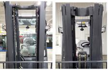
Nested I-beam mast rails provide the operator a wider view through the mast. Standard and multi-stage free-lift masts are available with lift heights up to 217-in.
