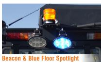
Many industrial operations require Blue (or other color) Spot Lights that project onto the floor. We offer "key-on" or "directionally activated" configurations. Amber safety beacon is standard.
