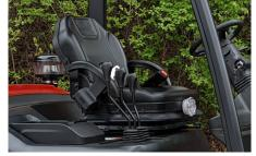
Comfortable full suspension seat adjust for operators up to 370-lbs. It features fore/aft/vertical travel, 20° pivoting backrest, OPS system, and orange seatbelt.
