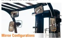
Multiple convex mirror configurations are utilized across the GT Series. These include interior and exterior mounting locations to assist the operator.
