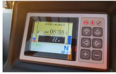
LCD display has integral engine protection system with alarm (monitors coolant temp, oil temp, and engine oil pressure). Speed control is also available.
