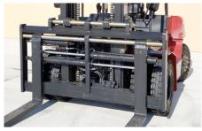
Pin-type and optional hook-type carriages are available. Side shift & hydraulic fork positioning will position forks without operator leaving the cabin.
