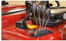
Ergonomic hydraulic control levers minimize driver fatigue and feature proportional control for precise load placement.
