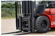
Multiple ISO hook-type carriages are available. Sideshift and hydraulic fork position carriages helps position forks without operator leaving the cabin.
