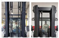
Nested I-beam mast rails provide the operator a wider view through the mast. Standard and multi-stage free-lift masts are available with lift heights up to 315-in.
