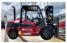
Lifting eyes are available across the GT Series. Mounted on the mast and rear chassis, they serve as proper lift points for lifting/lowering units into ships.
