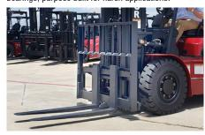
Multiple ISO hook-type carriages are available. Side shift and hydraulic fork position carriages helps position forks without operator leaving the cabin.
