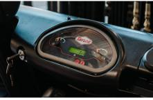
Dash display has integral engine protection system with alarm (monitors coolant temp, oil temp, and engine oil pressure). Speed control is also available.
