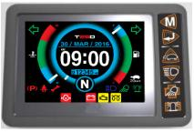
LCD display has integral engine protection system with alarm (monitors coolant temp, oil temp, and engine oil pressure). Speed control is also available.
