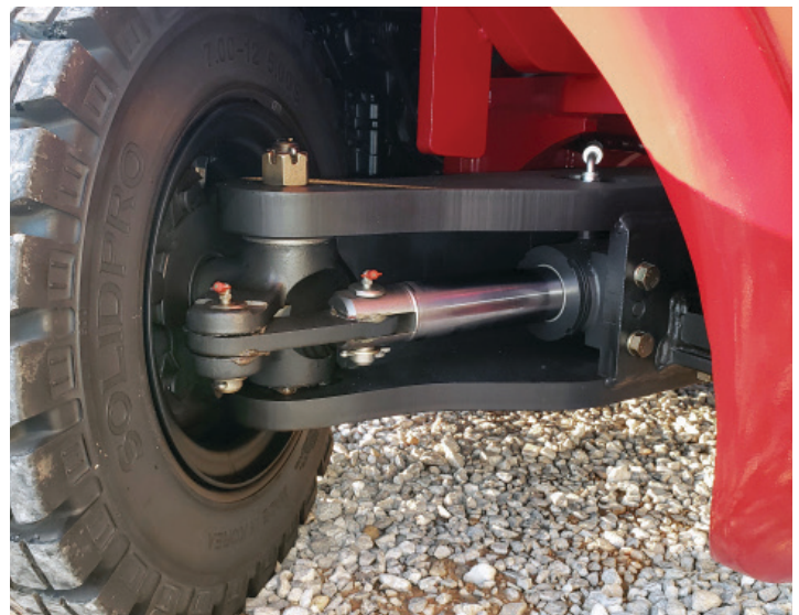
Heavy Duty Steer Axle Mounted on Rubber Isolators. Toughest Steer Axle Profile Available
