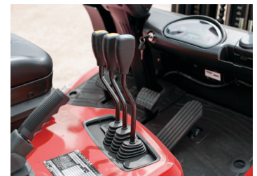
Hood Mounted Hydraulic Control Levers and Ratchet Style Hand Brake
