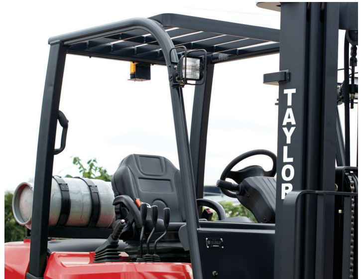
Isolation Mounted Open Operator Base with Overhead Guard Partial and Fully Enclosed Cabs Also Available (Optional)
