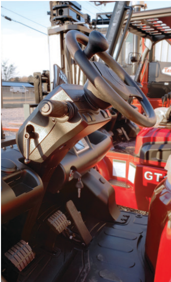
Adjustable Steering Column Pivots 30 Degrees
