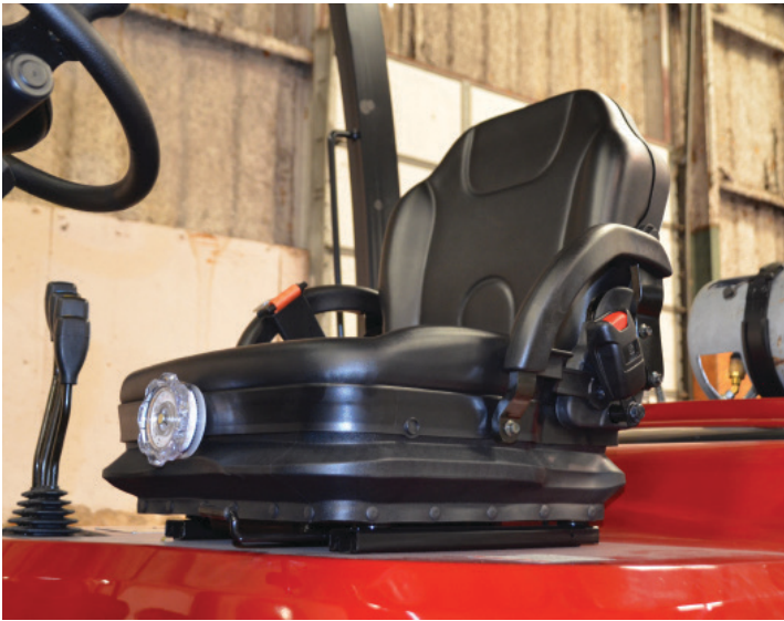
Adjustable Black Vinyl Mechanical Suspension Seat. Features Adjustable Weight Range
