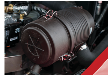
Donaldson Style Air Cleaner with Safety Element
