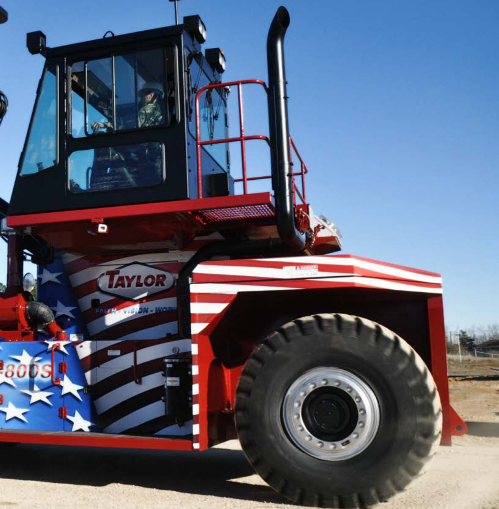
Featured truck in this picture is a: TXO-800S (Cap. 80,000-lbs at 48" L.C.)
