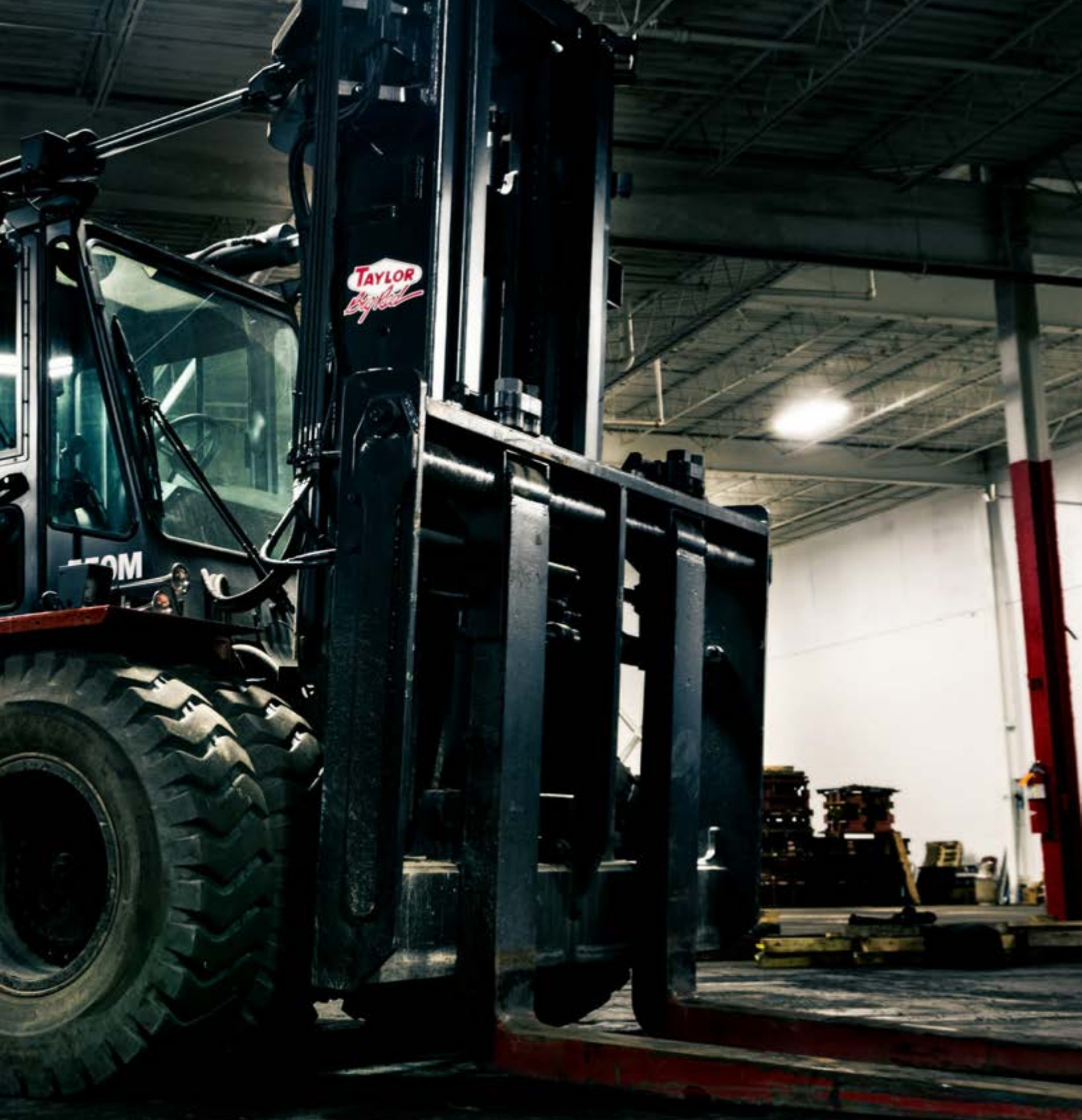
Featured truck in this picture is a: X-550M (Cap. 55,000-lbs at 48" L.C.)
