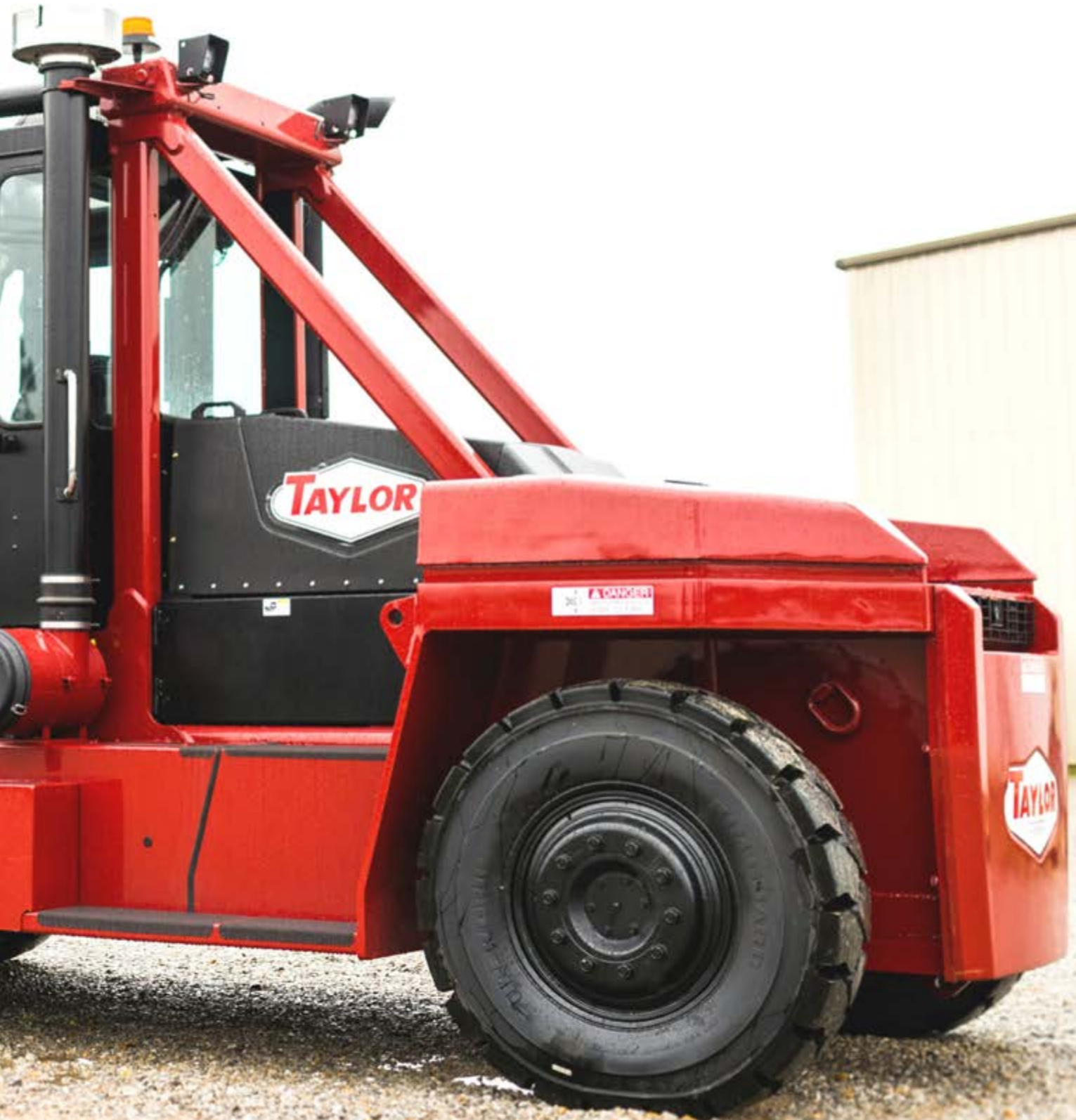
Featured trucks in this picture are: XH-350L (Cap. 35,000-lbs at 48" L.C.)
