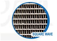
The Square Wave (cotton core style) radiator increases turbulent air which enhances non-clogging properties. Only available on trucks equipped with LPG engine.
