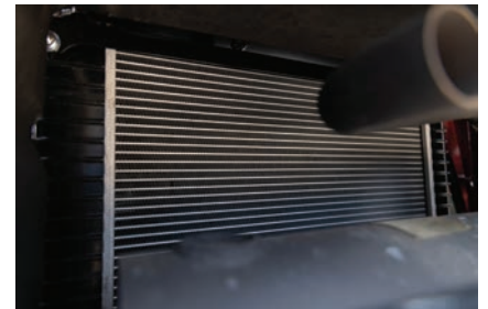
Open core copper radiator features corrugated fins with flat plate tubes. (4.6 fins per inch)
