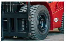
Single or Dual (drive tire) planetary front axles feature hydraulically actuated wet disc brakes. Available SOLID tires help prevent downtime due to flats.
