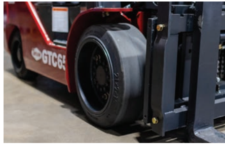
Single drive planetary front axles feature hydraulically actuated wet disc brakes. Polyurethane & non-marking cushion tires are also available.
