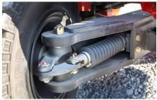
Steer axles endure heavy stress. GT steer axles feature fully boxed single cylinder design, with tapered roller bearings, purpose built for harsh applications.
