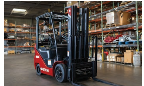
The available Vertical Mast System will stop the mast at the vertical position from ground when the truck is not in motion.
