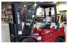
The partial cab option has front glass with windshield wiper, solid roof and sky-view window. This provides protection from the elements and retains ease of entry.
