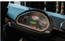
Dash display has integral engine protection system with alarm (monitors coolant temp, oil temp, and engine oil pressure). Speed control is also available.
