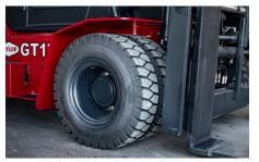
Dual drive tire planetary front axle features hydraulic actuated wet disc brakes. Available SOLID tires help prevent downtime due to flats.
