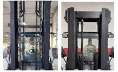
Nested I-beam mast rails provide the operator a wider view through the mast. Standard and multi-stage free-lift masts are available with lift heights up to 315-in.
