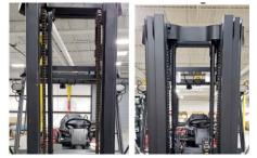
Nested I-beam mast rails provide the operator a wider view through the mast. Standard and multi-stage free-lift masts are available with lift heights up to 275-in.
