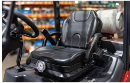
Comfortable full suspension seat adjust for operators up to 370-lbs. It features fore/aft/vertical travel, 20° pivoting backrest, OPS system, and orange seatbelt.
