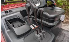
Ergonomic hydraulic control levers minimize driver fatigue and feature proportional control for precise load placement. Fingertip controls are also available.
