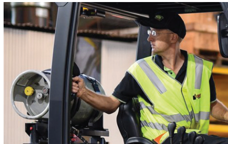
The GTC features a rear grab handle with a horn button to assist the operator in notifying anyone in the area of the machine's presence.
