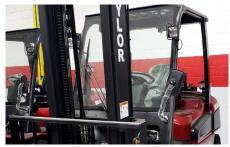
The partial cab option has front glass w/windshield wiper and solid roof w/sky-view window. It provides protection from the elements and retains ease of entry.
