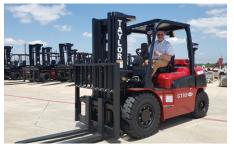
Working in containers introduces special height constraints. The available 87" reduced height overhead guard is purpose built for this low height application.
