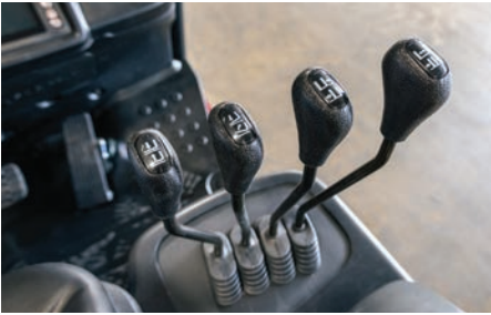
Ergonomic hydraulic control levers minimize driver fatigue and feature proportional control for precise load placement. (fingertip controls available)
