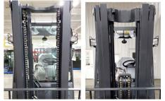
Nested I-beam mast rails provide the operator a wider view through the mast. Standard and multi-stage free-lift masts are available with lift heights up to 217-in.
