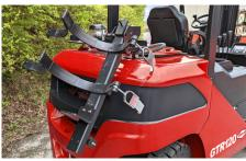
Changing LPG tanks can be difficult for some operators. The optional swing-out, drop-down tank bracket allows operators to load a tank with ease.
