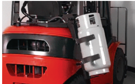
Changing LPG tanks can be difficult for some operators. The optional swing-out, drop-down tank bracket allows operators to load a tank with ease.
