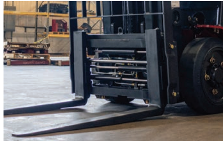
Multiple ISO hook-type carriages are available. Sideshift and hydraulic fork position carriages help position forks without operator leaving the cabin.
