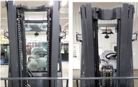
Nested I-beam mast rails provide the operator a wider view through the mast. Standard and multi-stage free-lift masts are available with lift heights up to 312-in.
