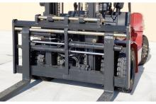
Pin-type and optional hook-type carriages are available. Side shift & hydraulic fork positioning will position forks without operator leaving the cabin.
