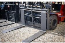
Multiple fork profiles are available. If something other than std. pallet forks is required, we can meet that need. (Special thin plywood/lumber forks shown).
